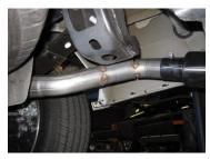
INSTALL EXIT PIPES # E & F ONTO TAILPIPES. ROTATE UNTIL LEVEL, USE CLAMP # H TO SECURE PIPES TOGETHER. DO NOT TIGHTEN.
