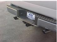
INSTALL YOUR STAINLESS TIPS TO YOUR DESIRED LOOK, THEN GO BACK AND TIGHTEN ALL CLAMPS. ROTATE SYSTEM FOR BEST CLEARANCE BEFORE TIGHTENING.
