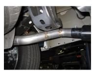
INSTALL EXIT PIPES # E & F ONTO TAILPIPES. ROTATE UNTIL LEVEL, USE CLAMP # H TO SECURE PIPES TOGETHER. DO NOT TIGHTEN.
