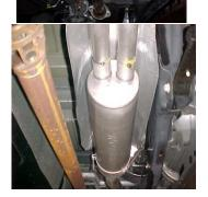
INSTALL MUFFLER # B ONTO HEADPIPE 1  $\frac{1}{2}$ " TO 2". USE CLAMP # G TO SECURE MUFFLER TO HEADPIPE. DO NOT TIGHTEN. USE A JACK STAND TO HOLD UP THE MUFFLER. OUTLETS SHOULD BE LEVEL.
