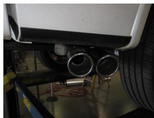
INSTALL YOUR STAINLESS TIPS TO YOUR DESIRED LOOK. NOW GO BACK AND TIGHTEN ALL CLAMPS FROM THE FRONT WORKING YOUR WAY BACK. AFTER YOU HAVE CHECKED FOR CLEARANCES GO BACK AND TIGHTEN ALL NUTS, BOLTS AND CLAMPS.
