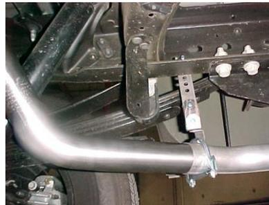
NEXT, INSTALL EXIT PIPES #E ONTO OVERAXLE PIPES. USE CLAMPS # I TO SECURE EXIT PIPE TO OVERAXLES. CUT EXIT PIPES TO DESIRED LENGTH..
