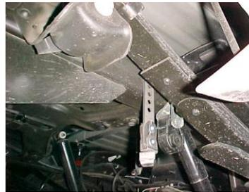
INSTALL PASSENGER SIDE OVERAXLE PIPE #C INTO MUFFLER 1 1/2" TO 2". USE CLAMP # I TO SECURE. DO NOT TIGHTEN. ROTATE UNTIL PIPE TOUCHES HANGER. USE CLAMP #I TO HOLD PIPE TO HANGER. DO NOT TIGHTEN.
