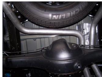
8. Install driver side overaxle tailpipe #G onto extension pipe, use clamp #J to secure pipe. Do not tighten. Insert welded hanger into rubber grommet.
