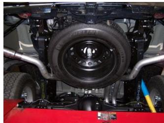
9. Next, install the exit pipes #H. Use clamps #J to secure the tailpipes.
