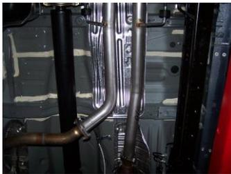
4. Install muffer #C onto headpipes 1.5"-2" with the louvers facing towards the converter. Use a jack stand to support the muffer. Use clamps #J to secure the muffer to the headpipes. Do not tighten. Muffer inlet is looking into the louvers.
