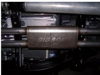
5. Install extension pipe #D into muffer. Use clamp #J to secure. Do not tighten. Next install driver side extension pipe #E into muffer using clamp #J to secure. Do not tighten. Insert welded hanger into rubber grommet.
