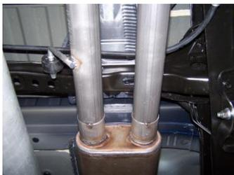
10. Install stainless steel tips. Clamp down. When you have everything in place, firmly tighten all bolts and clamps down securely. Use stainless steel cleaner and a Scotch Brite pad weekly to prevent tip from discoloration. Inspect all fasteners after 25-50 miles of operation and re-tighten as necessary.
