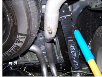
6. Install the passenger side overaxle tailpipe #F to the extension pipe. Use clamp #J to secure. Do not tighten. Insert welded hanger into rubber grommet.
