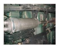
INSTALL MUFFLER #B ONTO THE HEAD PIPE 1-1/2" TO 2". OUTLETS SHOULD BE ON TOP, THEN INSTALL BAND CLAMP # H ONTO MUFFLER INSERT HANGERS INTO RUBBER GROMMETS.
