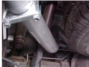
INSTALL DRIVER SIDE TAILPIPE #D INTO MUFFLER AT LEAST 1 1/2" TO 2". THIS PIPE WILL ROUTE OVER THE AXLE AND BETWEEN THE SHOCK AND TIRE. ATTACH CLAMP #G TO SECURE TAILPIPE TO MUFFLER. DO NOT TIGHTEN. INSERT WELDED HANGER INTO RUBBER GROMMET.
