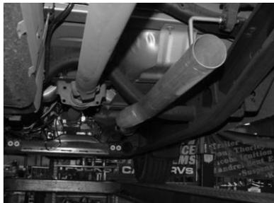
INSTALL PASSENGER SIDE TAILPIPE #C INTO MUFFLER AT LEAST 1 1/2" TO 2". USE CLAMP #G TO SECURE PIPE TO MUFFLER. DO NOT TIGHTEN. THE TAILPIPES WILL BOTH LEAN TOWARDS THE DRIVER SIDE LOOKING FROM THE REAR OF THE VEHICLE.
