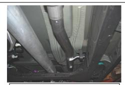
3. Install muffler assembly Item # B onto the head pipe 6". You may need to use a jack stand to support the muffler while installing the tailpipe. Use Item# E to clamp the muffler assembly to the head pipe. Loosely tighten down.
