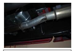
2. Install Head Pipe Item # A into the factory head pipe. Use the clamp Item # E at this connection. Loosely tighten down the clamp.
