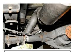
6. With proper clearance from spare tire install the exhaust tip onto the tailpipe. The system was designed to have the tip 1" below the quarter panel of the vehicle. With the tip in your desired position begin to tighten down all clamp connections from the front head pipe back.
