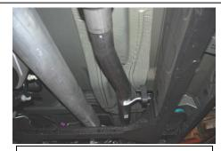
3. Install muffler assembly Item # B onto the head pipe. You may need to use a jack stand to support the muffler while installing the tailpipe. Use Item# E to clamp the muffler assembly to the head pipe. Loosely tighten down.
