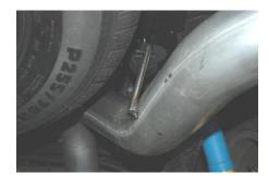
from the spare tire install the exhaust tip onto the tailpipe. The system was designed to have the tip 1" below the quarter panel of the vehicle. With the tip in your desired position begin to tighten down all clamp connections from the front head pipe back.
