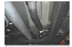
3. Install muffler assembly Item # B onto the head pipe. You may need to use a jack stand to support the muffler while installing the tailpipe. Use Item# E to clamp the muffler assembly to the head pipe. Loosely tighten
