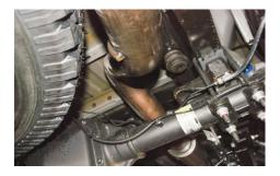
6. With proper clearance from spare tire install the exhaust tip onto the tailpipe. The system was designed to have the tip 1" below the quarter panel of the vehicle. With the tip in your desired position begin to tighten down all clamp connections from the
