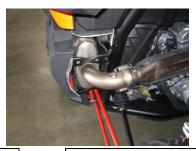
3. Next install the Gibson Muffler assembly. Install the top hanger mounts first then slide the inlet over the factory head pipe re using the factory gasket and springs. Once in position, install Headpipe and top muffler springs.
