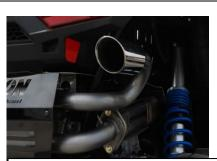
4. Next install the Gibson Muffler assembly. Install the top hanger mounts first then slide the inlet over the factory head pipe re using the factory gasket and bolts. Once in position, install Headpipe and top muffler springs.
