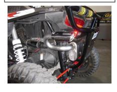
7. Once everything has been installed and tighten install your supplied Gibson tips. Slide the tips on to your desired look and tighten down. Check for 1" clearance and go have fun.
