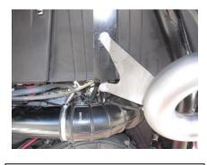
5. Bolt the tailpipe brackets to the rear under bed bracket. You will use Bolt Kit # B. Use the large fender washers on the back side of the top hole. You may have to loosen the factory bracket to adjust for fitment. Do not tighten until all bolts are installed. Install both sides.
