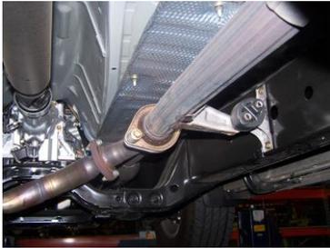
2. To remove the stock exhaust, unbolt the 2-bolt flange just in front of the muffler. Then cut your tailpipe off behind the muffler. Leave all rubber grommets on the factory hangers on the vehicle.
