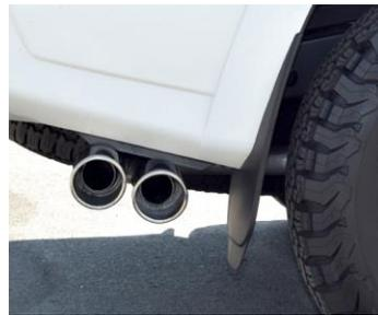
8. When you have everything in place, firmly tighten all bolts and clamps down securely. Use stainless steel cleaner and weekly to prevent tip from discoloration. Inspect all fasteners after 25-50 miles of operation and re-tighten as necessary.
