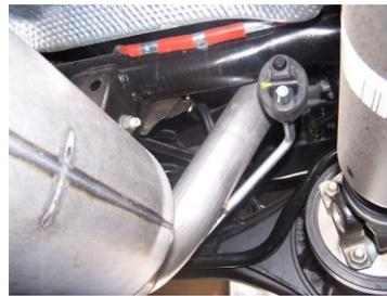
5. Install the over axle tailpipe #C into the muffler 1.5-2". Secure to the muffler using clamp #F. Do not tighten. Insert welded hanger into rubber grommet.
