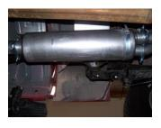
**3.** Install muffler #B onto head pipe #A  $1\frac{1}{2}$ "-2" with the louvers facing towards the converter. Use a jack stand to support the muffler. Use clamp #G to secure the muffler to the headpipe. Do not tighten. Muffler inlet is looking into the louvers.
