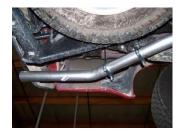
**7.** Next install the exit pipes #E. Use clamp #H to secure. DO NOT TIGHTEN.
