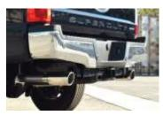
**8.** Install stainless steel tips. Clamp down. When you have everything in place, firmly tighten all bolts and clamps down securely. Use stainless steel cleaner weekly to prevent tip from discoloration. Inspect all fasteners after 25-50 miles of operation and re-tighten as necessary
