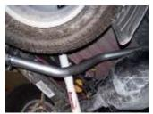
**6.** Install the driverside overaxle tailpipe #D into the muffler 1½-2". Use clamp #H to secure. DO NOT TIGHTEN. Rotate until it meets with the rubber grommet. DO NOT TIGHTEN.
