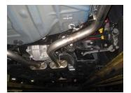
6. Install passenger side tailpipe/dual tip assembly #C. Insert all welded hangers into rubber grommets. Secure tailpipe with clamp #D. Do not tighten. Now go back and make sure the first two mufflers in the middle are level.
