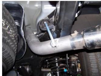
**8.** Install the exit pipe #E on the tailpipe. Secure together with clamp #F. Do not tighten. Roll the exit pipe until it is at the correct angle for your truck. Insert the welded hanger into rubber grommet.
