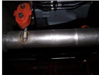
**6.** Install extension pipe #C into muffler 1½-2". Insert welded hanger into rubber grommet. Use clamp #F to secure to muffler. Do not tighten.
