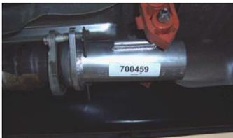
**4.** Attach head pipe #A onto your existing stock 2 bolt flange. Use bolt kit #H to secure it. Do not tighten. Insert welded hanger into rubber grommet.
