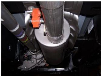
**5.** Install muffler #B onto headpipe 1½"-2" with the louvers facing towards the converter. Outlet will be at the 6 o'clock position. Use a jack stand to support the muffler. Use clamp #F to secure the muffler to the headpipe. Do not tighten. Muffler inlet is looking into the louvers.
