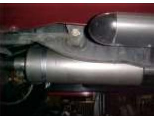
INSTALL MUFFLER # C ONTO YOUR RESONATOR 1 1/2" -2". USE CLAMP # I TO SECURE MUFFLER TO THE PIPE, DO NOT TIGHTEN.
