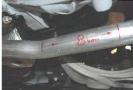
3. To remove the Passenger Side measure 8" down the pipe from the back of the muffler. Mark and cut with a hack saw or cut off wheel. Leave the factory rubber grommets in place they will be re used.
