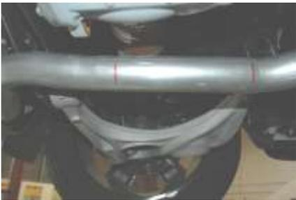
2. To remove the driver side exhaust measure 8" from the bend located under the rear end forward. Mark and cut with a hack saw or cut off wheel. Leave the factory rubber grommets in place they will be re used.
