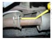
TO REMOVE YOUR STOCK EXHAUST, MEASURE 6" FROM THE 2-BOLT FLANGE LOCATED IN FRONT OF YOUR STOCK MUFFLER AND CUT.
