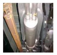
INSTALL HEADPIPE # A INTO STOCK PIPE. THE END OF THE PIPE SHOULD BE AT THE 12 O'CLOCK POSITION, ATTACH WITH FACTORY CLAMP. DO NOT TIGHTEN. INSERT WELDED HANGER INTO RUBBER GROMMET. REMOVE THE HANGER FRO THE FRAME & RELOCATE TO THE HOLES JUST TO THE LEFT OF THE OTHER HOLES YOU WILL NEED TO PRY THE INSERTS OUT & RE-INSTALL SEE PHOTO
