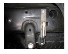
5. Next install drivers side rear hanger and grommet with bolt kit on the outside of the driver side frame rail. Use the factory drilled hole just forward of the large hole seen in the photo above.
