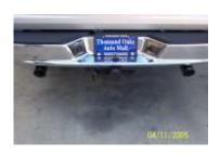
Install the exit pipes #E. Use clamps #J to secure exit pipes to the tailpipes. Rotate the exit pipe to the best fit for your vehicle.
