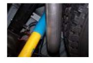
7. Slide the driver side over axle tailpipe #D into the muffler 1.5-2". Use clamp #H to secure tailpipe to muffler. Do not tighten. Insert welded hangers into rubber grommets.
