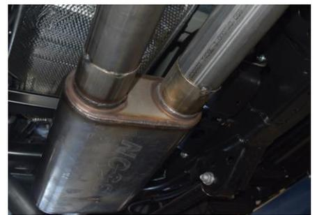
4. Install the Gibson Muffler with Logo facing downward. Use jackstand to support muffler Do not tighten until final install.
