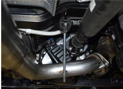
3. Install your Driver side head pipe #A using the factory Gasket and supplied bolts in Item #K and install your Passenger side headpipe. Do not tighten until final install.
