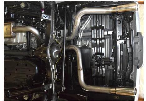
7. After each connection has been tighten go back and double check your tip positions as things can change with each connection being tighten. Use a stainless cleaner weekly to maintain the polished finish of the tips.
