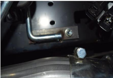
5. Install the hanger Item# I on the passenger side frame rail using the existing hardware that supported the OEM wiring harness bracket. Install rubber the hanger. Now Install the overaxle pipe into the outlet of the muffler. Note the long section of the pipe will go in the muffler outlet. Do not tighten.
