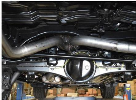
6. Install the Y-pipe Item # E with the long portion of the Y pipe heading to the Passenger side. Install both exit pipes. With everything in place adjust the kit to obtain the proper clearance. Minor adjustments make big changes so take your time. Install the Gibson Tips. Begin to tighten exhaust starting at the front flange connections.
