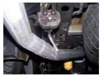
6. Remove spare tire to install tailpipes (Reference vehicle manual for removal of spare tire). Now install Driver side tailpipe #D into the muffler 11/2-2". Use clamp #H to secure tailpipe to muffler. DO NOT TIGHTEN. Insert welded hangers into rubber grommets.
