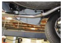
7. Install Passenger side tailpipe #C into the muffler 11/2-2". Use clamp #H to secure tailpipe to muffler, DO NOT TIGHTEN, Insert welded hangers into rubber grommets.
