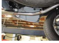
8. Install the exit pipes #E. Use clamp #H to secure exit pipes to tailpipes. DO NOT TIGHTEN. Rotate pipes to adjust for desired look. Reinstall spare tire.
