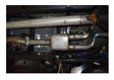
Install muffler onto head pipe # A 1-1/2" to 2". Use a jack stand to support the muffler. Use clamp #H to the secure the muffler to the head pipe. Do not tighten
