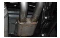
Install head pipe # A onto you're existing stock pipe using Clamp #H to secure connection. Use a jack stand to support the factory exhaust. Do not tighten.
