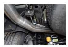
Install the driver side tailpipe # D into the muffler at least 1-1/2" to 2". This pipe will route over the axle and between the Frame rail and tire. Use clamp # H to secure pipe to the muffler. Do not tighten. Insert hangers into rubber grommet.
