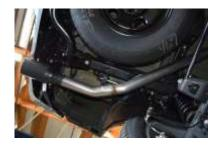
Install the Gibson Tips onto your exit pipes. Place the tips to your desired position. Be for tightening down the system it is recommended to secure the tips the position you want and check the location after each connection is tightened.
