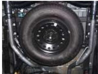
8. Install exit pipes #E onto tailpipes. Cut to your preferred length then use clamps to secure exit pipes to tailpipes. Install stainless steel tips. Clamp down.
