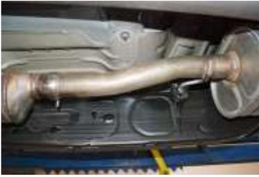
2. To remove stock exhaust, un clamp it at the connection behind the Y-pipe. Make sure to leave all rubber grommets in the factory location. **You will re-use stock clamp.** For easier removal of exhaust, cut behind the muffler. Use WD-40 to remove hangers from grommets.
