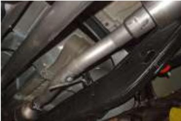
3. Install Headpipe #A onto your factory headpipe using your stock clamp. Install the hanger into the rubber grommet and do not tighten until install is complete.
