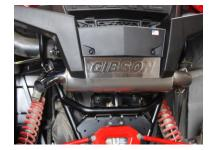
**GIBSON EXHAUST** systems are designed on a factory stock vehicle. Any aftermarket products installed could increase the sound levels of the exhaust. **Make sure there is a 1**" clearance from ALL rubber brake lines, shock boots, lines, tires, etc. to
