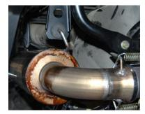
5. Install the factory gasket onto the original header.
