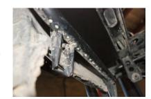
4. Install Item# E. You will need to remove the two factory torx screws located on the rear of the vehicle pictured below. They are located directly below the "POLARIS" logo. Install the heat shield with the long portion facing towards the rear of the vehicle protecting the plastics above the rear heat shield.
