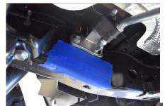
5. Slide the second supplied 2.5" band clamp over the headpipe then slip your new Gibson muffler onto the headpipe, tighten aluminum hangers into their locations with the 4 factory bolts.
