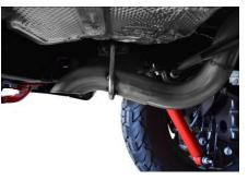
8. To install your XT Tip simply remove the exhaust from the Gibson head pipe and re install the tip using the same clamp and driver side only hanger. Protect your tips when in storage. We do not want any dings or dents.
