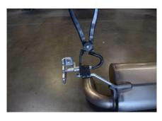
4. Remove hangers from OEM exhaust using removal pliers or large channel pliers and re-install them on the Gibson as shown. Using a lubricant can aid in the removal.
