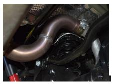
3. Once you have removed the OEM exhaust install Item# E onto the factory oem pipe. Use clamp # b to secure. Be sure notch is lined up and do no tighten clamp.
