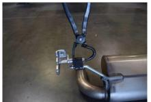
4. Remove hangers from OEM exhaust using removal pliers or large channel pliers and re-install them on the Gibson as shown. Using a lubricant can aid in the removal.
