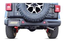
7. Adjust the tip to your preference. Make sure everything is clear of frame rails and parts and re tighten the system starting from the front clamp. Check everything after each clamp is tightened.
