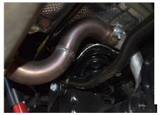
3. Once you have removed the OEM exhaust install Item# E onto the factory oem pipe. Use clamp # b to secure. Be sure notch is lined up and do no tighten clamp.
