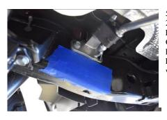
5. Slide the second supplied 2.5" band clamp over the headpipe then slip your new Gibson muffler onto the headpipe, tighten aluminum hangers into their locations with the 4 factory bolts.
