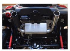
Slide the 2.5" band clamp over the expanded part of the muffler and make clamp snug but not tight. Install the Gibson provided tips. Check for exhaust clearance before tightening.
