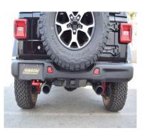
Adjust the tips to your preference. Make sure everything is clear of frame rails and parts and re tighten the system starting from the front clamp. Check everything after each clamp is tightened.
