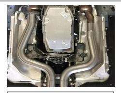
2. Install the PS headpipe Item A and Item B onto the factory pipes. Reuse the factory gaskets and hardware. Do not tighten. Keep loose until final fitment. Install 02 sensor at the end of the install.
