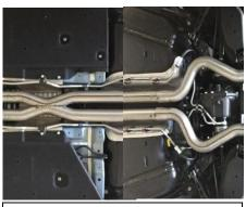
3. Install Item C onto the headpipes using clamps Item I to secure. Do not tighten. Install Item D & E onto the X pipe. Keep everything loose.
