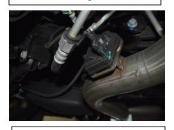
7. Remove the NPT valves from your factyory exhaust located on the tailpipes. Using your 10MM, install both onto your mid pipes and re connect. Re install your Factory O2 sensor. It may take 4-500 miles for your vehicle to fully adjust to the changes in exhaust flow.
