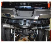
7. Install both the driver side and passenger side exit pipes. Use a jack stand to support the tips up while you make final adjustments to find the perfect fit. Adjust the kit to fit properly giving at least 1.5" of clearance from all components. Begin to tighten the system from the frot forward. Be sure after each connection is tightening to go back and check your tip position as it can move.
