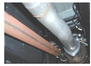
3. Install headpipe #A onto your existing stock front pipe Re-using the factory nuts.
