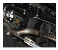
4. Install the Extension Y-pipe #B onto headpipe 1.5"-2". Use clamp #G to secure. Do not Tighten
