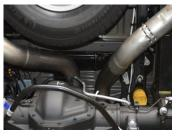
5. Install the overaxlepipe pipes. The Driverside will have the NPT bung for the factory sensor. Do not tighten. This is a critical part in the exit location of your exhaust tips. If you are having troubles getting the tips to exit even this is the point where adjustments made can help find your perfect fit.
