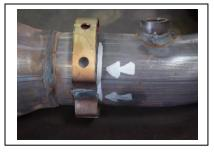
3. Once head pipe is removed mark and cut the pipe just behind the heat shield bracket closest to the catalytic convertor. (see image for reference) deburr all cuts.
