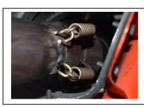
6. "clock" ghost pipe to allow proper positioning for springs to reinstall. When in proper positioning tighten band clamp bolts.
