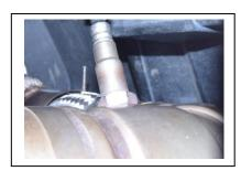
7. Reinstall O2 sensor and OEM clamps to head pipe. Re use the factory gasket.
