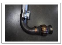
4. Slide band clamp on loosely giving both stock head pipe and ghost pipe equal space in the band clamp.
