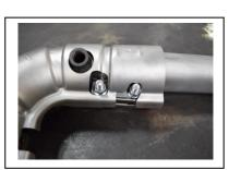
8. If you are reinstalling OEM heat shield you will need to modify heat shield to allow for band clamp bolts clearance. It is recommended that you always use the factory heat shield.
