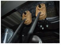
**4.** INSTALL OVERAXLE TAILPIPE # C INTO THE OUTLET OF THE MUFFLER 1<sup>1</sup>/<sub>2</sub>" TO 2". INSERT WELDED HANGERS INTO THE FACTORY RUBBER GROMMET. USE CLAMP #E TO ATTACH THE OVERAXLE PIPE TO THE MUFFLER OUTLET. DO NOT TIGHTEN.
