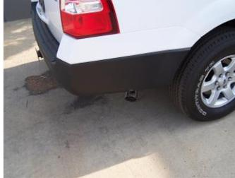
**11.** Install stainless steel tip. Clamp down. When you have everything in place, firmly tighten all bolts and clamps down securely. Use stainless steel cleaner and a Scotch Brite pad weekly to prevent tip from discoloration. Inspect all fasteners after 25-50 miles of operation and re-tighten as necessary
