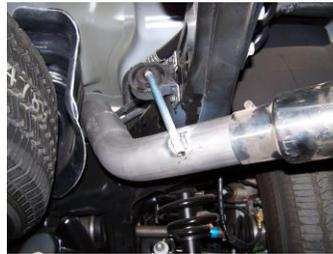
**8.** Install the exit pipe #D on the tailpipe. Secure together with clamp #E. Do not tighten. Roll the exit pipe until it is at the correct angle for your truck. Insert the welded hanger into rubber grommet.
