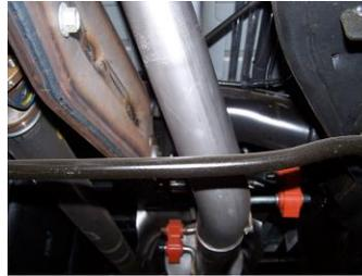
**7.** Install the over axle tailpipe #C into the extension pipe 1 1/2"-2". Use clamp #E to secure. Do not tighten. Insert welded hanger into the rubber grommet.
