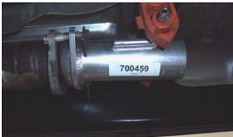
**4.** Attach head pipe #A onto your existing stock 2 bolt flange. Use bolt kit #G to secure it. Do not tighten. Insert welded hanger into rubber grommet.
