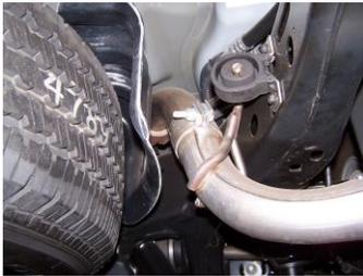
**3.** For easier removal of the stock exit pipe, remove rear hanger from the frame. Then remove exit pipe and re-install stock rear hanger.
