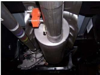
**5.** Install muffler #B onto headpipe 1 1/2"-2" with the louvers facing towards the converter. Outlet will be at the 6 o'clock position. Use a jack stand to support the muffler. Use clamp #E to secure the muffler to the headpipe. Do not tighten. Muffler inlet is looking into the louvers.
