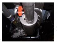
**5.** Install muffler #B onto headpipe 1½"-2" with the louvers facing towards the converter. Outlet will be at the 6 o'clock position. Use a jack stand to support the muffler. Use clamp #F to secure the muffler to the headpipe. Do not tighten. Muffler inlet is looking into the louvers.
