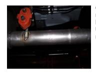
**6.** Install extension pipe #C into muffler 1½-2". Insert welded hanger into rubber grommet. Use clamp #F to secure to muffler. Do not tighten.
