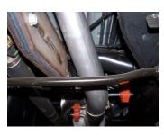
**7.** Install the over axle tailpipe #D into the extension pipe 1½-2". Use clamp #F to secure. Do not tighten. Insert welded hanger into the rubber grommet.
