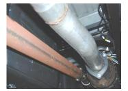
4. Install headpipe #A onto your existing stock front pipe Re-using the factory nuts.
