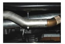
2. INSTALL HEADPIPE #A ONTO THE FACTORY EXTENSION PIPE. INSERT WELDED HANGER INTO RUBBER GROMMET. USE CLAMP #E TO ATTACH IT TO THE FACTORY EXTENSION PIPE. DO NOT TIGHTEN
