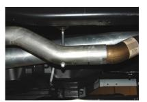
2. INSTALL HEADPIPE #A ONTO THE FACTORY EXTENSION PIPE. INSERT WELDED HANGER INTO RUBBER GROMMET. USE CLAMP #E TO ATTACH IT TO THE FACTORY EXTENSION PIPE. DO NOT TIGHTEN
