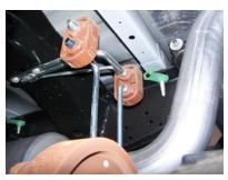
4. INSTALL OVERAXLE TAILPIPE # C INTO THE OUTLET OF THE MUFFLER 1<sup>1</sup>/<sub>2</sub>" TO 2". INSERT THE REAR WELDED HANGER INTO THE FACTORY RUBBER GROMMET. USE CLAMP #E TO ATTACH THE OVERAXLE PIPE TO THE MUFFLER OUTLET. DO NOT TIGHTEN.
