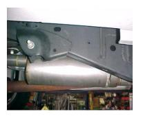
INSTALL MUFFLER # B ONTO HEADPIPE  $1\frac{1}{2}$ " TO 2". USE CLAMP # E TO SECURE MUFFLER TO HEADPIPE. DO NOT TIGHTEN. USE A JACK STAND TO HOLD UP THE MUFFLER. MUFFLER INLET IS LOOKING INTO THE LOUVERS. OUTLET SHOULD BE AT T HE 10 O'CLOCK POSITION.
