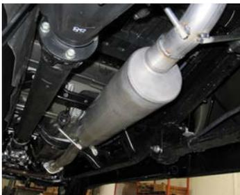
INSTALL MUFFLER #B ONTO HEAD PIPE 1-1/2" TO 2" WITH THE LOUVERS FACING TOWARDS THE CONVERTER. THE MUFFLER OUTLET SHOULD BE POSITIONED THE MUFFLER OUTLET SHOULD BE POSITIONED AT 12:00. USE A JACK STAND TO SUPPORT THE MUFFLER. USE CLAMP #E TO SECURE THE MUFFLER TO THE HEAD PIPE. DO NOT TIGHTEN. MUFFLER INLET IS LOOKING INTO THE LOUVERS.
