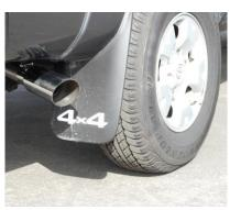
ALUMINMUM OR STAINLESS STEEL CLEANER TO POLISH YOUR TIP. MAKE SURE YOU HAVE A MINIMUM OF A 1" CLEARANCE ON ALL PIPES FROM ALL RUBBER BRAKE LINES, TIRES, SHOCKS, FUEL LINES, ETC. THEN TIGHTEN ALL CLAMPS AND HANGERS
