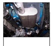
**3.** Install muffler #B onto head pipe 1½"-2" with the louvers facing towards the converter. Use a jack stand to support the muffler. Use clamp #F to secure the muffler to the headpipe. DO NOT TIGHTEN.
