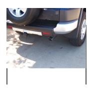
**6.** Install stainless steel tip #E. Clamp down. When you have everything in place, firmly tighten all bolts and clamps down securely. Use stainless steel cleaner and a Scotch Brite pad weekly to prevent tip from discoloration.
