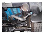
**5.** Next, install the exit pipe #D. onto overaxle pipe. Use clamp #F to secure to the tailpipes. DO NOT TIGHTEN. Insert welded hanger into rubber grommet.
