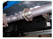
**1.** To remove the stock exhaust remove it from the 2-bolt flange located in front of the stock muffler. Disengage the welded hangers using WD-40 from the OEM rubber grommets. Do not damage or remove the rubber grommets as you will re-use them to mount your new system. Now, cut off tailpipe and remove exhaust.
