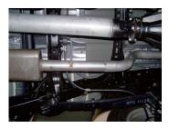
5. Install rear extension pipe #D onto muffler. Insert welded hanger into rubber grommet. Use clamp #H to secure the pipe. Do not tighten.
