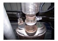
2. Remove the stock exhaust at the 2-bolt flange located in front of the muffler. Disengage the welded hangers from the OEM rubber grommets. Use WD-40 to help in the process. Do not damage or remove the rubber grommets as you will reuse them to mount your new system. Now, unbolt the tailpipe and remove exhaust. Do not throw away stock flange bolts, as you will reuse them.
